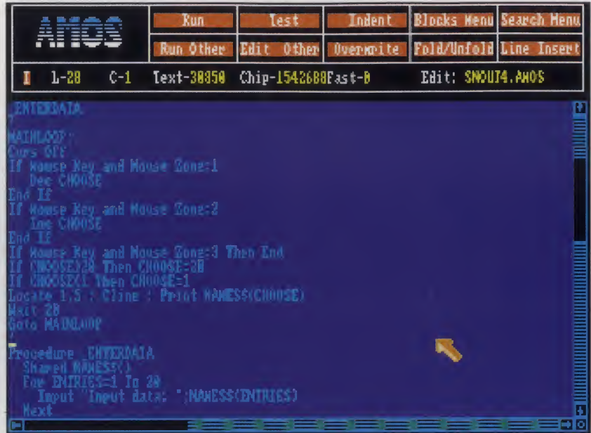
Here's the main loop of the code, the bit that checks which buttons have been clicked on. Once a Zone has been set up, it's so easy to find out what the person using your programs has selected - and it's much friendlier than relying on the keyboard.
